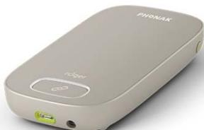
The Roger Multimedia Hub can be connected to any multimedia device used in the classroom ranging from smartboards and TV's to computers and videos. Roger Multimedia Hub can also be connected as a standalone media transmitter by an individual student for listening to an audiobook, a tablet or a lesson on a computer.
