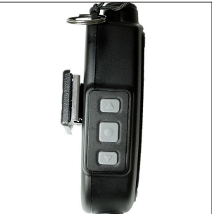
Volume +/- function and loudspeaker mute button when nexus accessories are used
